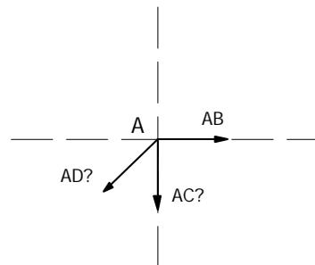
$$\Rightarrow AD = \sqrt{2}P \sin \alpha + 2\sqrt{2}P \cos \alpha \quad \text{et} \quad AC = -2P \cos \alpha - P \sin \alpha$$
