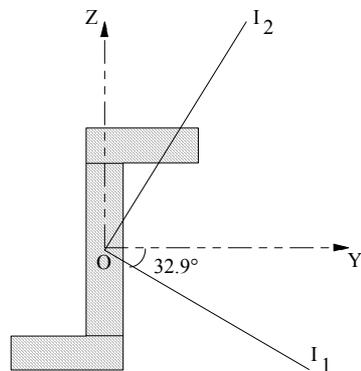
$$Z_G = \frac{\sum z_i S_i}{\sum S_i} = \frac{105 \times 360 \times 30}{3 \times 120 \times 30 + 360 \times 30} = 52.5 \text{ mm}$$
